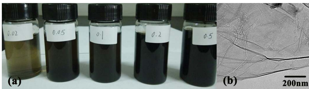
Figure 1. Photographs of (a) 9 wt % PVA aqueous solution with GO concentrations from 0.02 to 0.5 wt %, (b) TEM images of the GO sheets. [Color figure can be viewed in the online issue, which is available at wileyonlinelibrary.com .]
